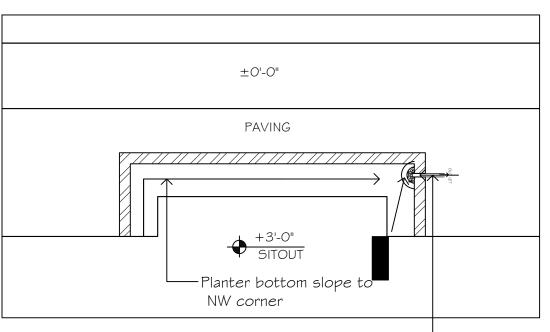
Drain outlet 2" Ø PVC pipe fixed@ in side planter FFL level .with slope towards outside pipe to have nelton mosquito cover on either side covering the opening THIS DRAWING IS THE PROPERTY OF M/S K.B.CONSULTANTS HYD.AND IS NOT TO BE COPIED OR USED WITHOUT PRIOR PERMISSION.
