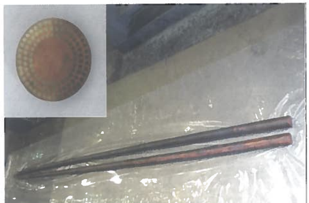
As Extruded 50 mm Dia rod of Nb-Cu
