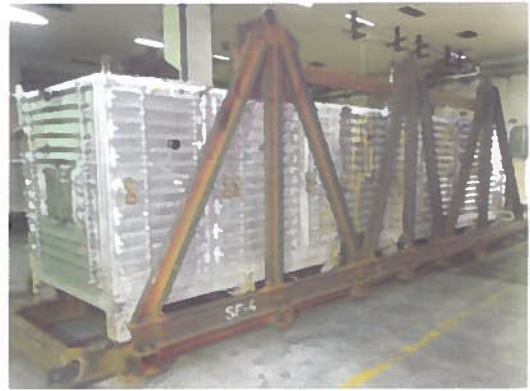
High Capacity Sintering Furnaces with Lifting Structure
