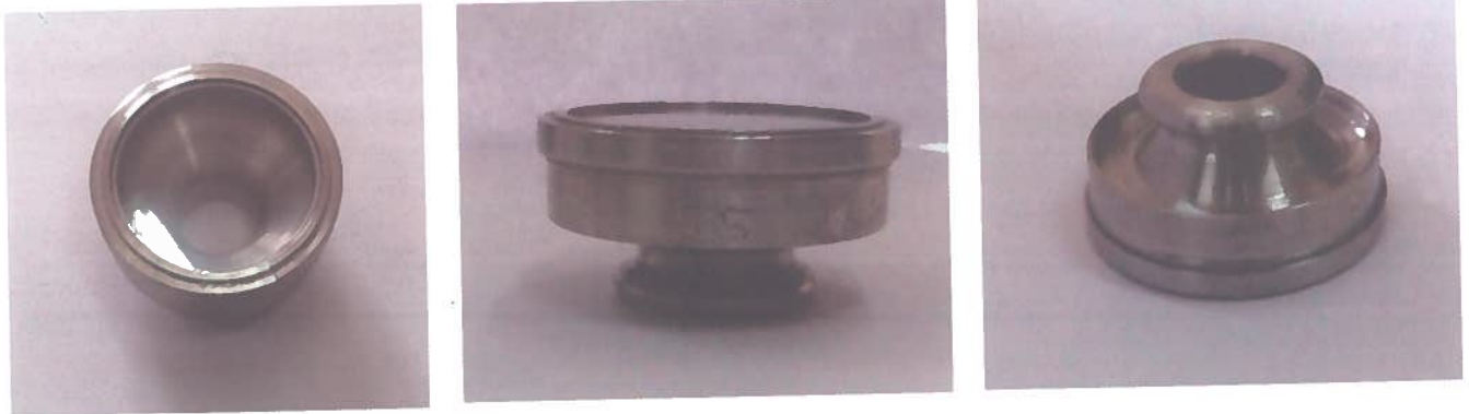
Different Views of In-house Fabricated SS Liquid Sample Holder of XRF Instrument
