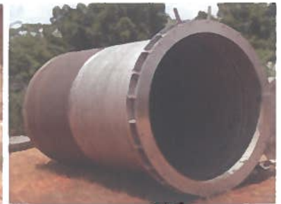
Vacuum distillation retort 1500Kg batch
