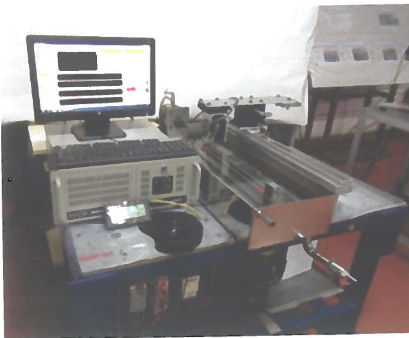
Prototype Automated Ultrasonic testing machine for PHWR end cap weld evaluation
