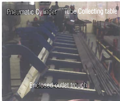
Automatic tube unloading unit
