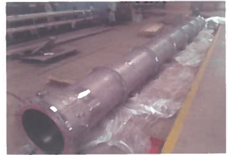
SS 310S Hot Chamber for Horizontal Vacuum Annealing
