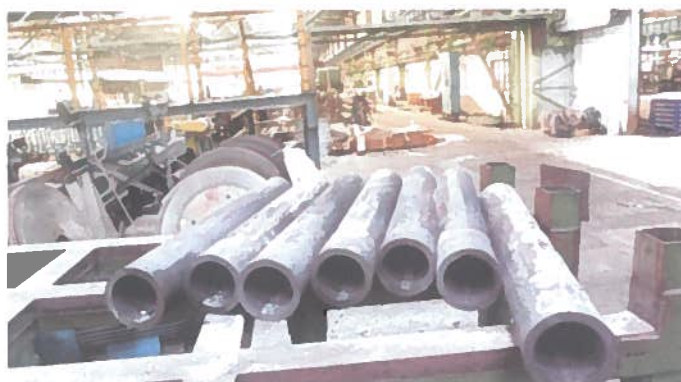
MDN 350 alloy hot finished tubes of size Ø222 OD x178 mm ID
