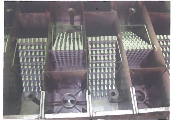
Innovative Coalescer in Stripping Section
