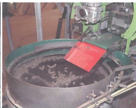
Automated Pellet Unloading System
