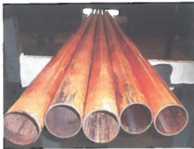
95 mm OD x 5.2 mm WT X 6.2 m L As extruded Zr-2.5% Nb PT Blanks for 220Mwe PHWR Tube
