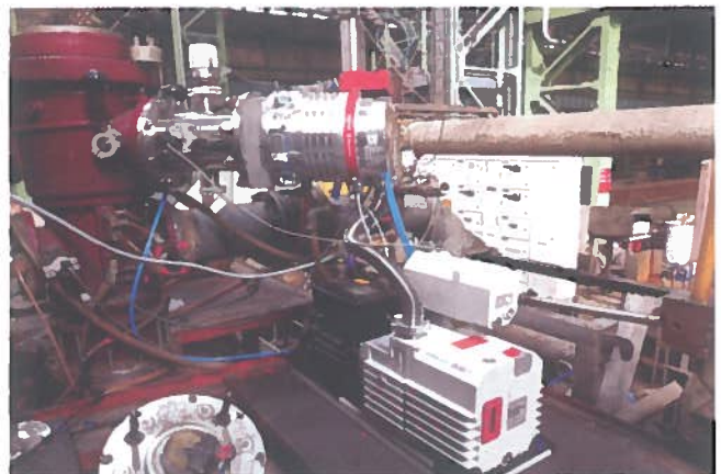
New vacuum system with Turbo molecular pump for cathode chamber
