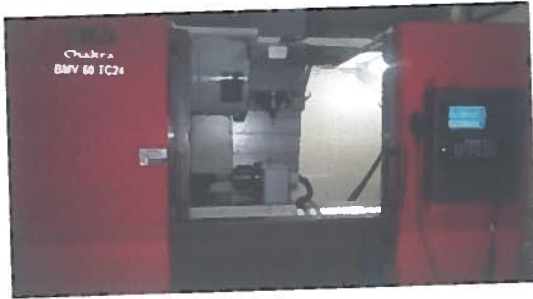
4-axis CNC Vertical Milling Centre stroke length of 1050mm (X-axis) x610mm (Y-axis) x610mm (Z-axis) equipped with rotary table (A-axis) for manufacture of pilger-mill dies and support plates.
