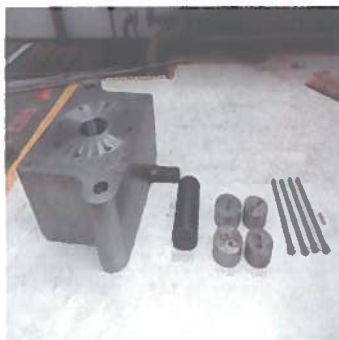
Die House for 2000 Te press ( After modification.)
