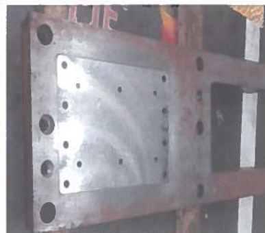
Die House for 2000 Te press ( After modification.)
