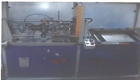
Modified end cap welding machine
