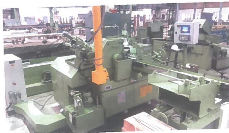
Centre-less grinder for HPT mandrel grinding with adjustable feed stands for accommodating the rods ranging from 2-25mm diameter and 350 and 400 mm in length to cater requirement of mandrels required for production of small diameter tubes for the manufacture reactivity mechanism assemblies and for strategic applications
