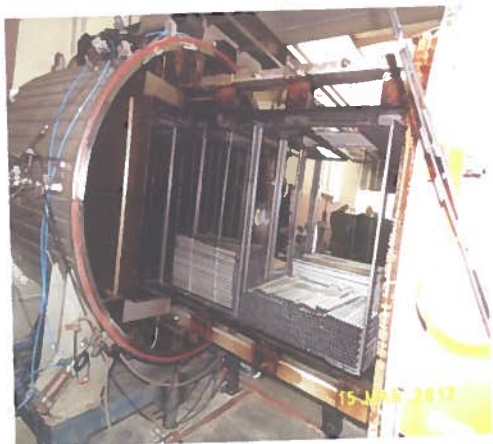
Loading of the VBF-III furnace with class-B tubes.
