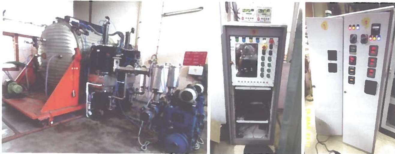
Re-commissioned vacuum baking furnace at NUFAP
