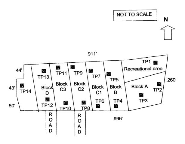
Fig. 1. Layout Plan for Residential Buildings at Nagaram, Keesara (M), showing locations of trial pits.
