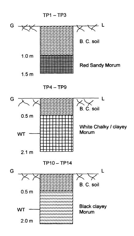
Fig. 2. Typical Logs of Trial Pits (TP) – Nagaram.
