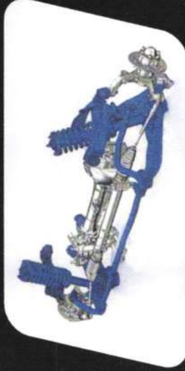
Front independent double wishbone suspension Heavy duty suspension for superior comfort and unmatched on-road durability.
