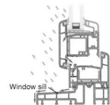
Casement system with Sill-Bottom drainage (S-3000) Figure - 2
