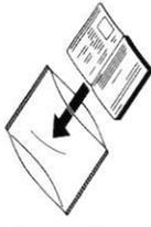
Set the feed selection lever to Bypass mode and load the document facing downward.
