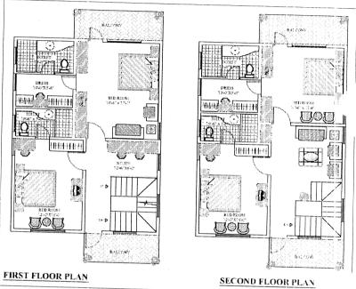
GROUND FLOOR BUILT UP AREA = 900,00 SFT FIRST FLOOR BUILT UP AREA = 1050,00 SFT SECOND FLOOR BUILT UP AREA = 1050,00 SFT TOTAL BUILT UP AREA = 3000,00 SFT PORTICO AREA = 246,00 SFT
